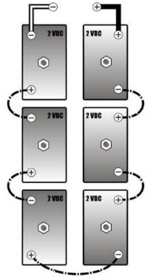
Figure 4.3: 24-volt battery configurations
