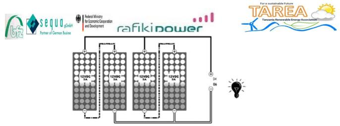
Figure 3.5: PV modules in series and parallel
