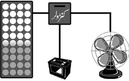
Figure 5.1: Controller in a PV system
