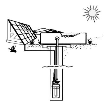
Figure 9.2: Solar water pumping system
