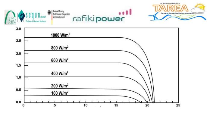
Figure 3.7: Effect of sunlight intensity on module performance (12VDC nominal)
