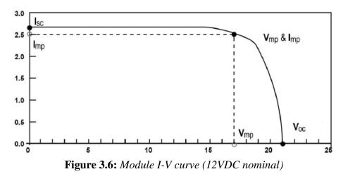
Figure 3.6 shows a typical I-V curve. Voltage (V) is plotted along the horizontal axis. Current (I) is plotted along the vertical axis. Most I-V curves are given for the standard test conditions (STC) of 1000 watts per square meter sunlight (often referred to as one peak sun) and 25 degrees C (77 degrees F) cell temperature.
