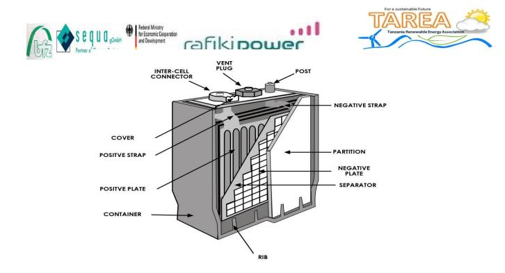
Figure 4.1: Cut-away of a standard lead acid battery cell
