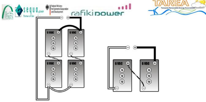
Figure 4.4: 48-volt battery configurations
