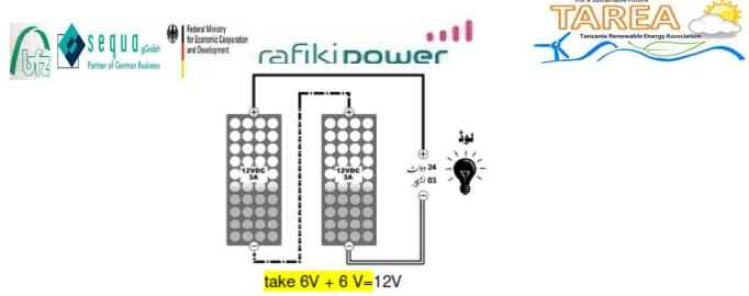
Figure 3.3: PV modules in series
