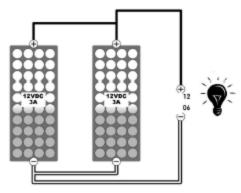
Figure 3.4: PV modules in parallel
