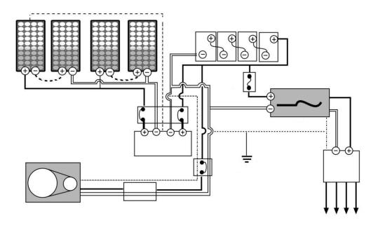
Figure 9.3: Hybrid system with generator
