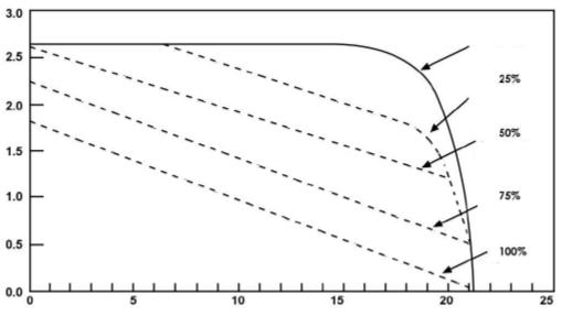
Figure 3.9: Effect of shading on module performance (12VDC nominal)
