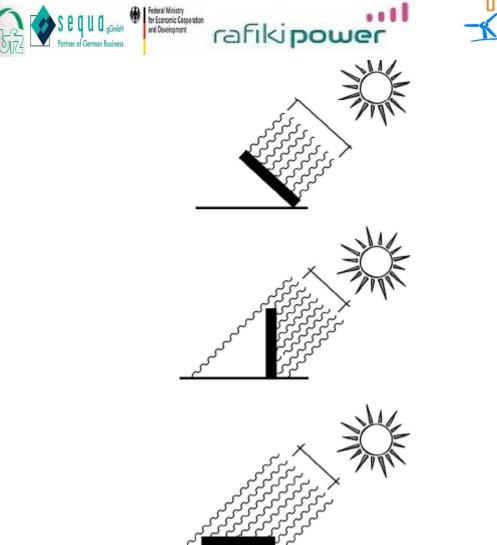
Figure 2.2: Effect of tilt angle
